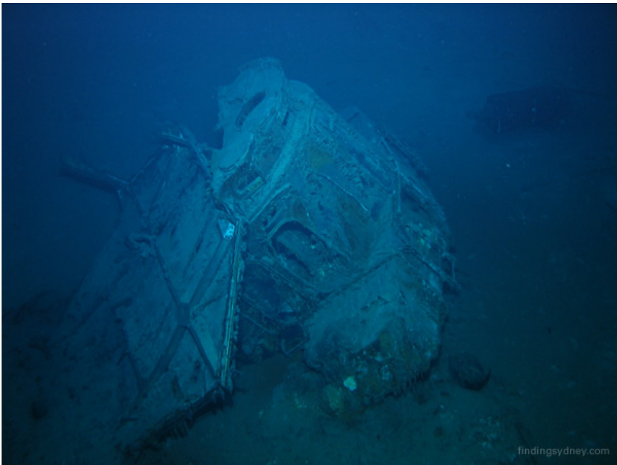
Above Photograph: The distinctive bridge deck head (roof) lying against the front of the Director Control Tower.
